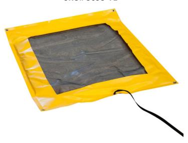
Dripillow Berms are engineered to be the ideal portable, outdoor drip and leak protection. They feature absorbent pads sewn into a UV resistant mesh for protection from the elements. These pads are placed inside a tough, industrial fabric shell to prevent excessive spills from reaching the ground. Welded in sandbags prevent the product from flipping over due to the wind, and the retrieval strap doubles as a cinch when folded for convenience and portability.
